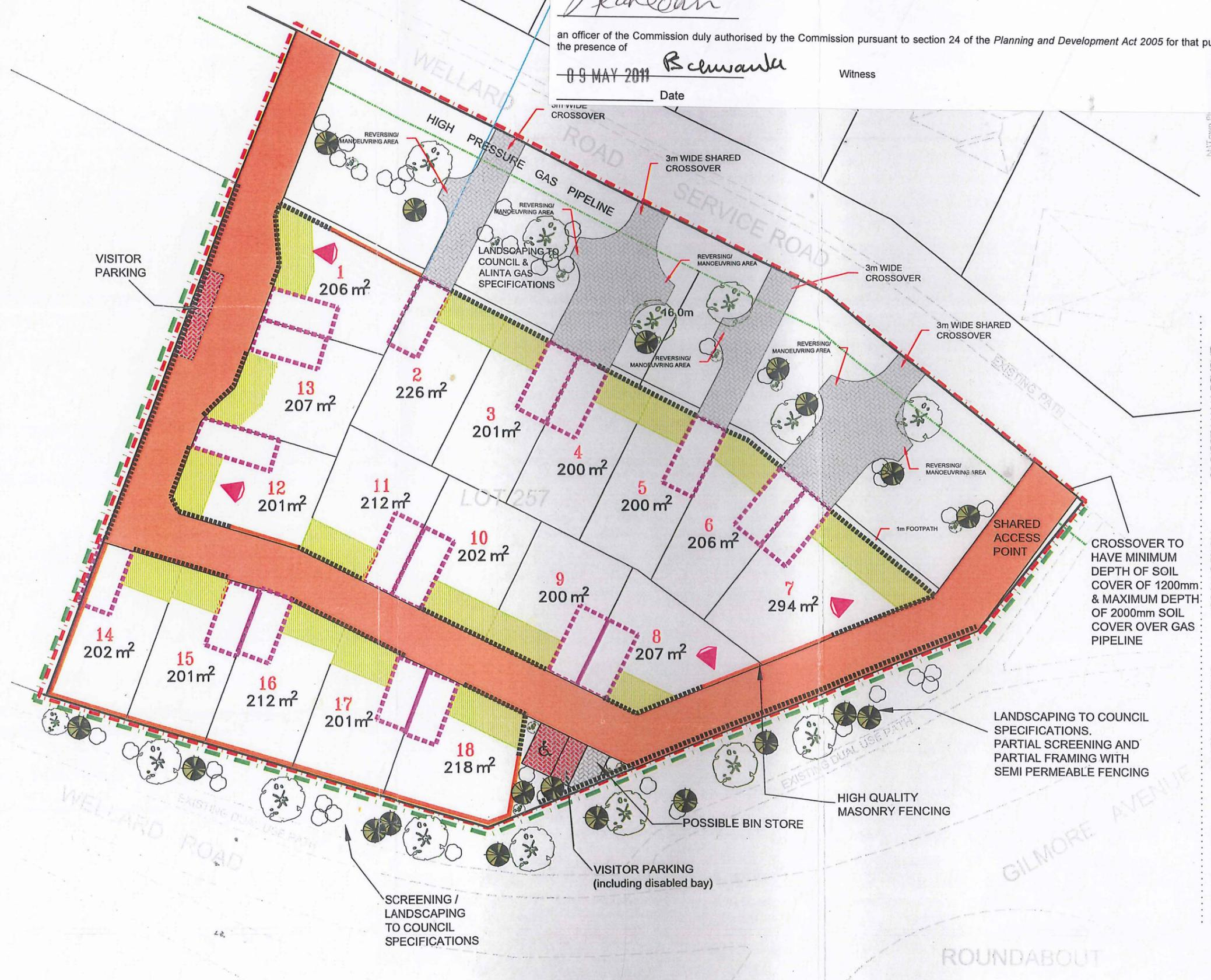
CROSSOVER TO HAVE MINIMUM DEPTH OF SOIL COVER OF 1200mm & MAXIMUM DEPTH OF 2000mm SOIL COVER OVER GAS PIPELINE
